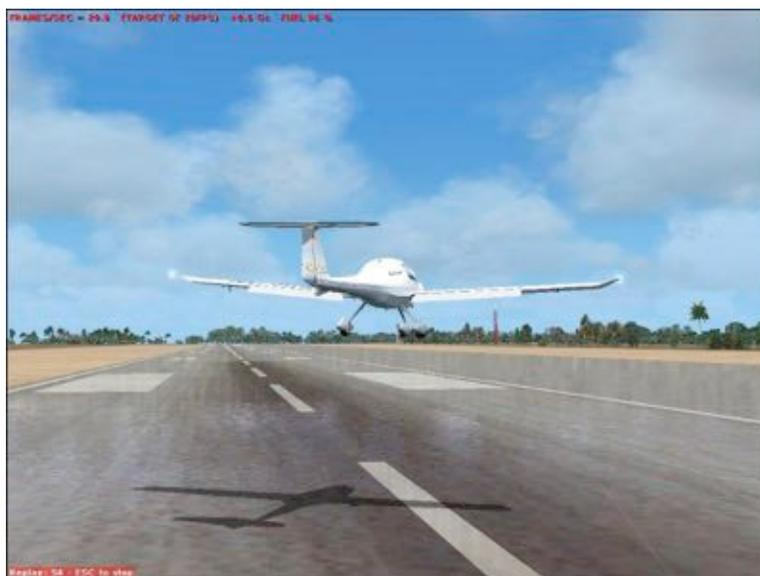
**Slip** - This describes the condition of flight when the flight controls are used in an uncoordinated fashion. For example, right rudder is depressed but the yoke is rolled to the left. Desired ground track is obtained by varying the bank angle and/or rudder pressure. Unlike the Crab, if flight controls are released, the aircraft will not maintain this condition.
