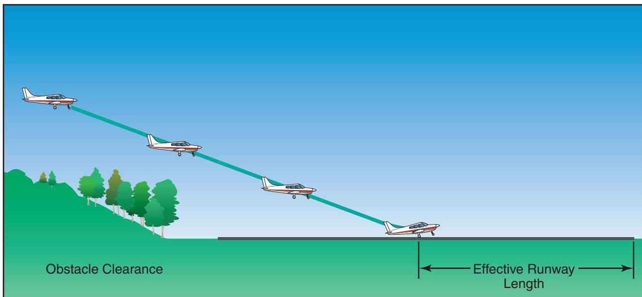
Figure 8-20. Landing over an obstacle.
